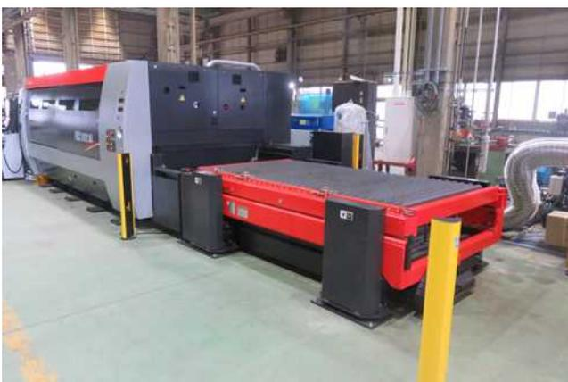
Installation of the "Fiber Laser" cutter
