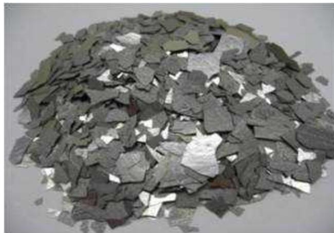
Photo: Flakes of neodymium iron boron alloy produced by strip casting method
