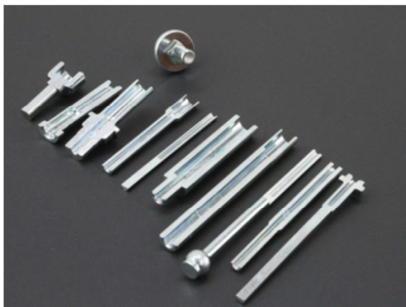
Photo: Vertically sliced samples of primary-processed products made by cold forging (after the plating process)
