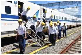
Frequent earthquakes, unpredictable fires in train cars, sudden train accidents—Techno Ace Ltd. has developed the Super Quick Ladder, an emergency escape ladder for railway vehicles that enables passengers to escape from a train promptly and safely in such emergency cases. The results of research conducted by the Railway Technical Research
